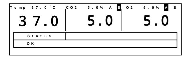
2. The CO<sub>2</sub> gas supply line will be switched from cylinder B to A
